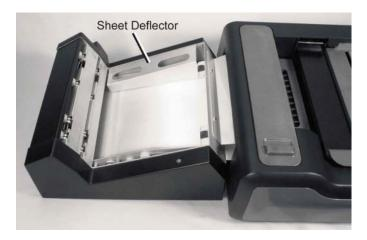
3. Mount the select stacker (lower) tray to the Select Stacker. The metal hooks go into the slots in the Select Stacker.
