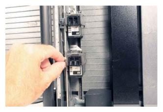
6. Move the printer to the desired position and lightly tighten the thumbscrew.
