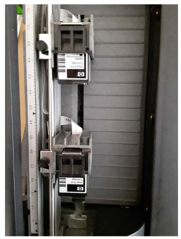
6. Move the printer to the 2.5 inch mark and lightly tighten the thumbscrew.
