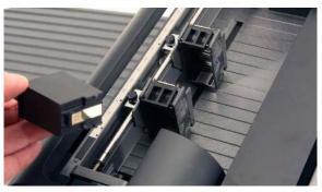
3. Using a clean swab, gently wipe the area of the cartridge holder that contains the electrical contacts.
