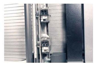
7. If your scanner is equipped with dual printers, adjust the position of the second printer.
