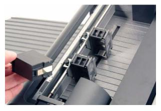
Slide the cartridge into the cartridge holder "feet first" then press the top of the cartridge firmly into the cartridge holder until you feel two clicks. This ensures that the cartridge is fully seated.
