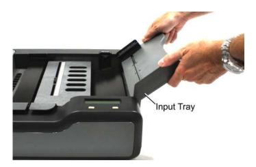
4. Insert the *Quick Tips* guides (shipped with your scanner) into the slot on the underside of the input tray. This helps prevent loss of the instructions.
