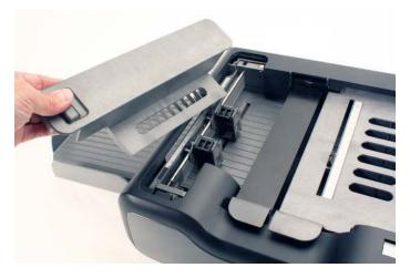
2. Note the location of the cartridge holder inside the printer assembly. Also note the ruler, printer alignment mark, and thumbscrew that sits beside the cartridge holder. These are the elements used to position the printer.
